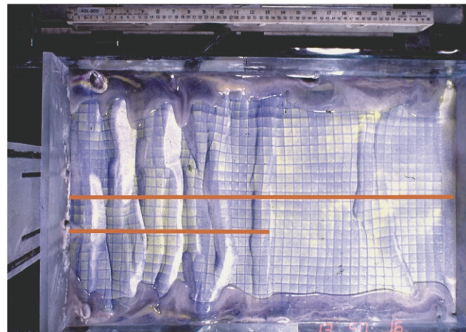
Fig. 4. Overhead photographs of models with two silicone décollements. Solid lines indicate cross-section locations for Figs. 5 and 6. The maps are lit from the right side (foreland), so slopes dipping to the right appear bright and those dipping to the left appear dark. The pushing wall for the model is on the left-hand side as it is in all cross-sections. (a) Model 327: 5 mm/h, (b) Model 330: 10 mm/h, (c) Model 339: 50 mm/h, (d) Model 323: 100 mm/h.
